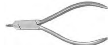
018-1029 Loop forming pliers Four steps beak for making precision loops of 3.45 or 6mm in round or rectangular wires. One tip is serrated to prevent wire slippage
