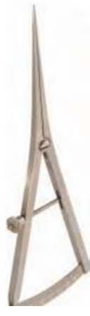
020-1132 Measuring Loop straight length 175 mm, measuring range 0 - 40 mm,
