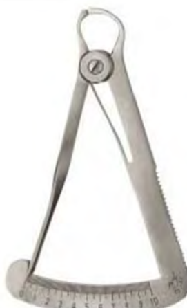
020-1134 Fig 2 Iwanson spring caliper For wax.
