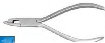
018-1030 Loop forming pliers with replaceable 440 stainless steel tip, three step tip has 1.14, 1.52 and 1.91mm diameters
